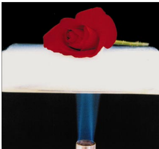
Figure 1. Aerogels have excellent insulating properties, as shown here for a silica aerogel tile.
